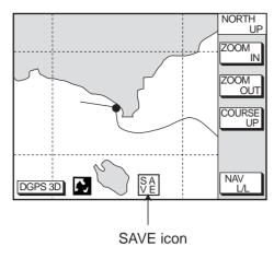
Figure 6-9 SAVE icon appearance on the plotter display
